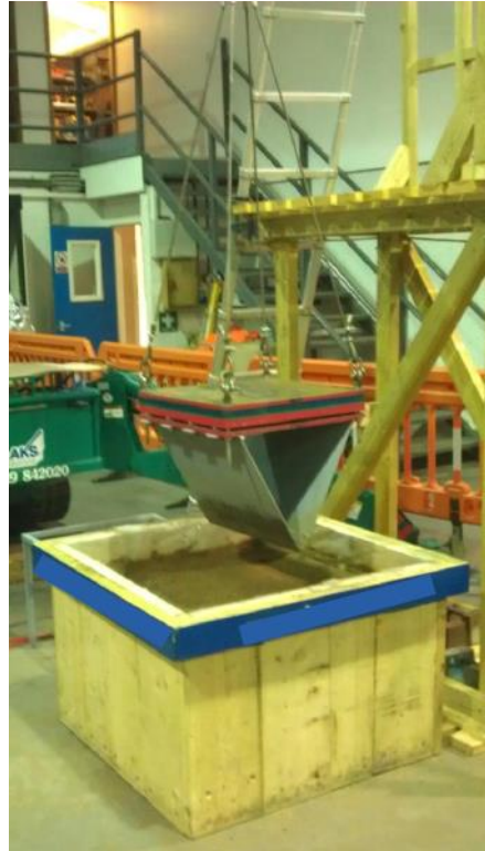
Figure 2. Drop Test Fixture As Described In Protocol 1 (Protocol 1 2014)
